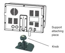
Installation of U-support bracket:
